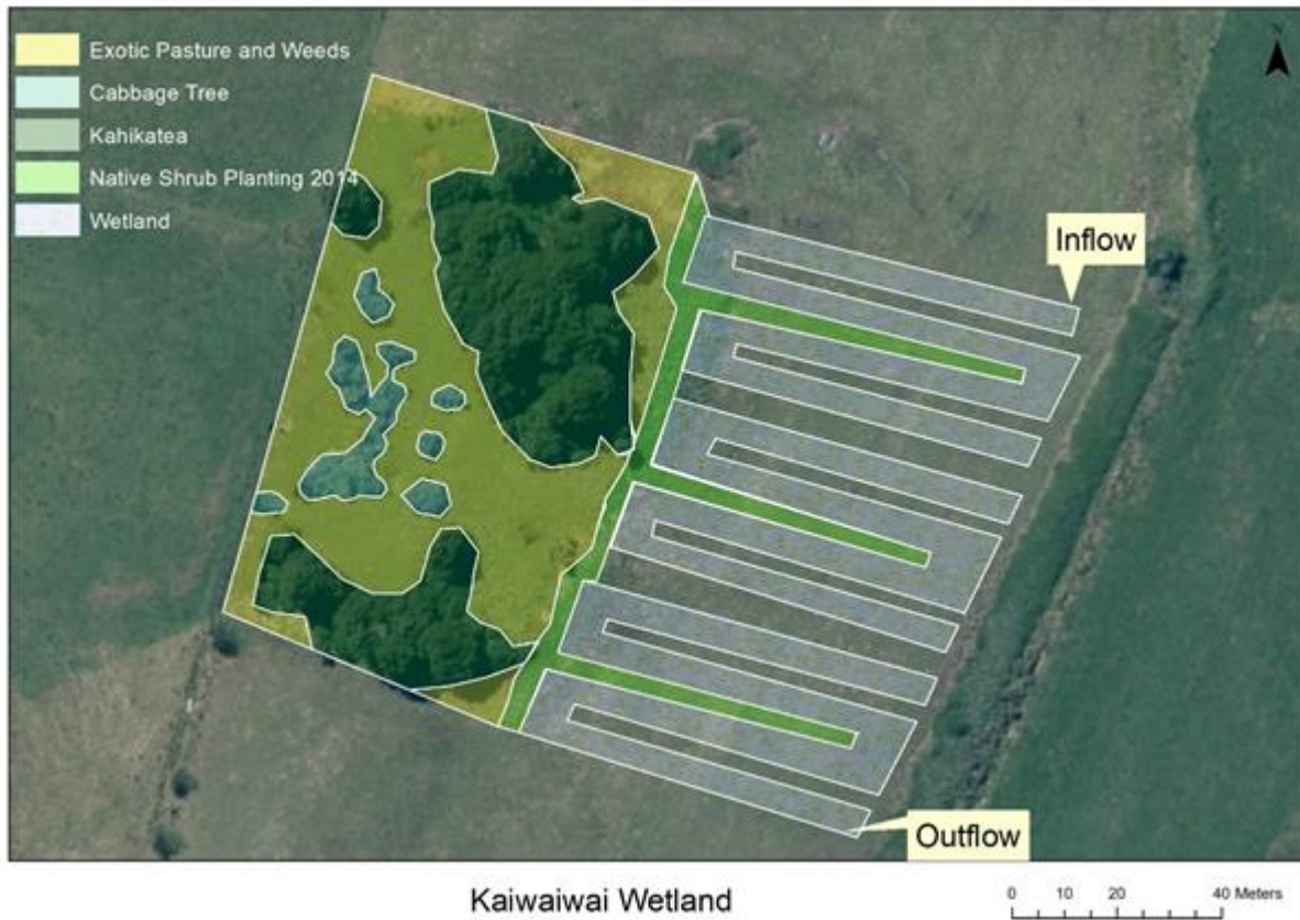
Figure 1 Map showing location remnant bush and design of wetland with entry and exit points.
