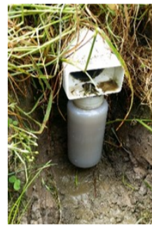
The first one litre of run-off from the catch-drain fills the sample bottle.
