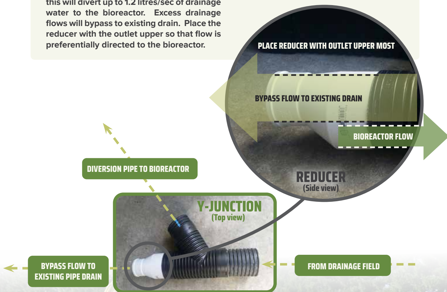
FIGURE 3 Arrangement of “Y” junction with 100 to 65mm reducer
